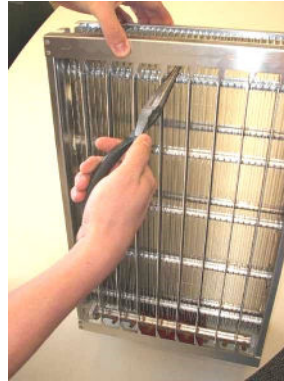
FIGURE 5 – INSTALL NEW IONIZER WIRES BY HOOKING EYELETS OVER THE SPRING CONNECTORS.
