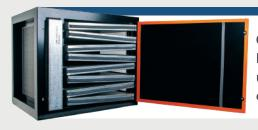
Odor control modules, optional for both AUTOCLEAN® and SMOKEMASTER® F72 PCUs can be customized to meet various airflow requirements. These modules utilize multi-stage re-fillable or replaceable filters, available in both activated carbon or potassium permanganate, to effectively adsorb odors.
