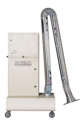
The M33V from Air Quality Engineering, Inc. is a self-contained media air cleaning system designed for use in source capture applications where mobility is desired. The M33V can be ordered in a three-stage filtration configuration which will effectively remove a broad range of airborne contaminants including fine dust, smoke, soot, vapors, mist, VOC's and more at a rate of up to 1250 CFM.
