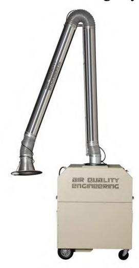
The new portable cartridge system from Air Quality Engineering Inc. is a complete self-contained media air cleaner for use in source capture applications in industrial settings. The Porta Air captures airborne contaminants such as welding smoke, grinding dust, plastic dust and other fine particles.
