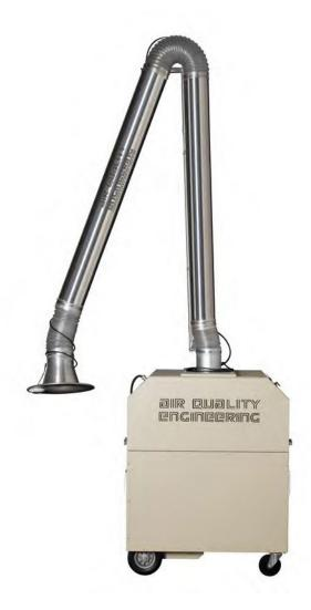
The new portable cartridge system from Air Quality Engineering Inc. is a complete self-contained media air cleaner for use in source capture applications in industrial settings. The Model AQE2000 captures airborne contaminants such as welding smoke, grinding dust, plastic dust and other fine particles.
