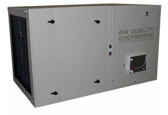
The M68 is a self-contained HEPA air cleaner rated at 99.97% efficient @ 0.3 microns. The M68 is designed for use where higher efficiency filtration is required and is intended for general background air cleaning applications. The M68 is rated for airflows up to 1850 CFM.
