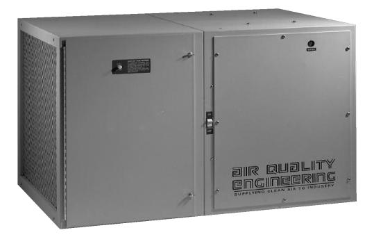
The F66 from Air Quality Engineering, Inc. is a self-contained electronic air cleaning system designed for general background cleaning applications. The F66 efficiently captures a broad range of airborne contaminants including smoke, fumes, soot, light dust and coolant mists at a rate of up to 2,600 CFM, with no costly filter replacement.
