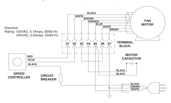
Single Phase Schematic (7 Wire Fan Motor)
